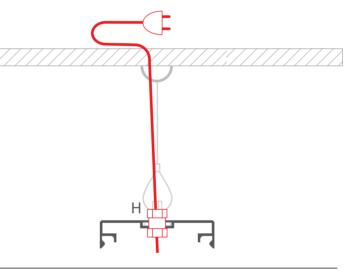
**11.** Assemble the extrusion (B) with the mounting strip (A). Connect the LED strips and run the cable through the gland to the power supply.
