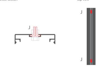
$\boldsymbol{9}_\bullet$  Suspend the mounting strip (A) using the hangers (J) and a chosen suspension system.
