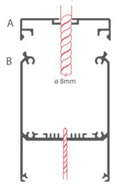
**2.** Bevel the channel in the mounting strip (A) over the gland hole. The drill bit diameter must be 12.5-14 mm. This will ensure correct mounting of the gland.
