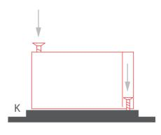
**5.** Insert the power supply bracket (K) in the extrusion (B).
