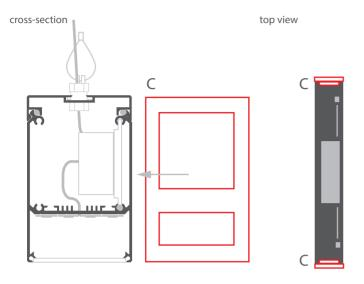
**14.** Put the brackets (D) in the hollows of the gaskets (C) and tighten them with the bolts (F).
