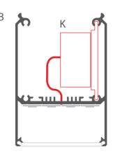
**6.** Secure the power supply bracket (K) by inserting one 2.4 mm plastic rod (M) into the guides on each side. Cut the rods to the required length. Next secure the rods with M3 pressure screws (O), tightening them with the Allen wrench to a min. depth of 2 cm.
