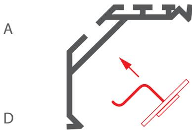
**4.** Connect power, then mount the extrusion in the drilled holes using springs.
