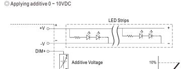
"DO NOT connect "DIM- to -V"
